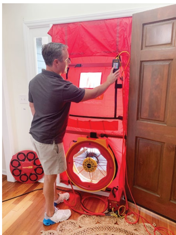
A blower door test being conducted to determine envelope leakage.
