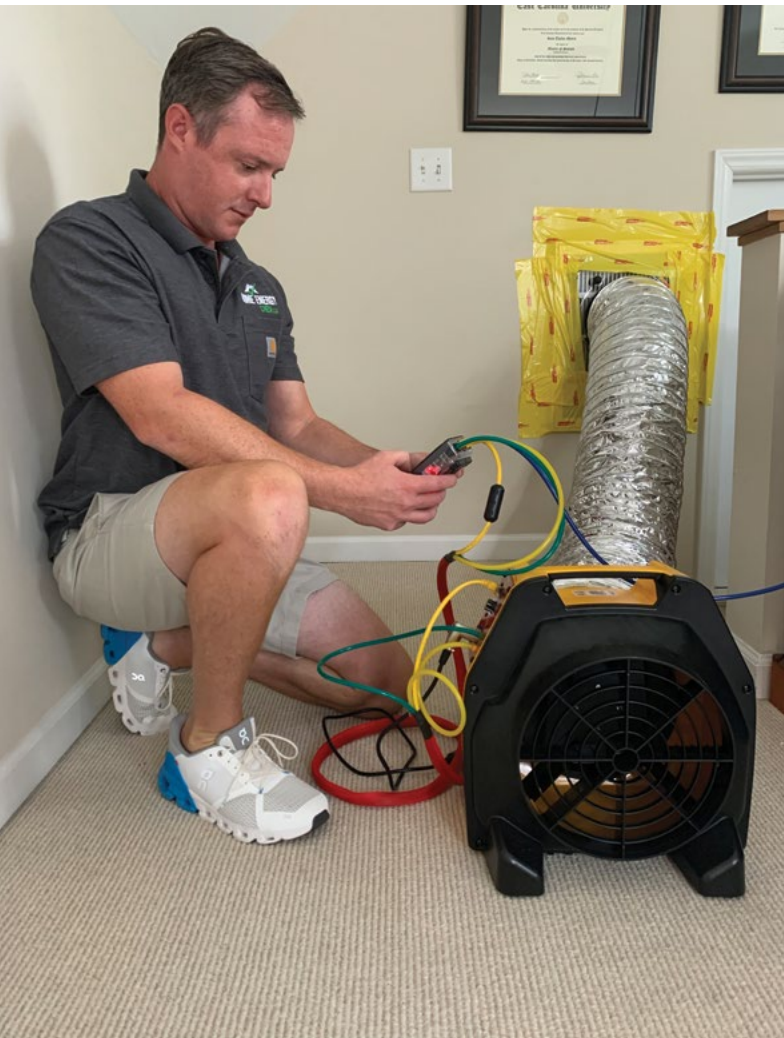
A duct system being tested for leakage.
