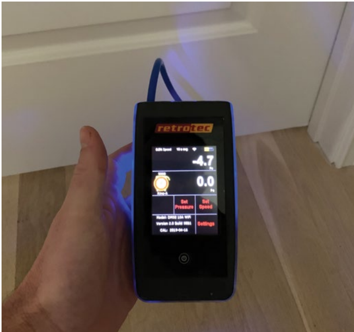
A high-precision manometer reading room pressure.
