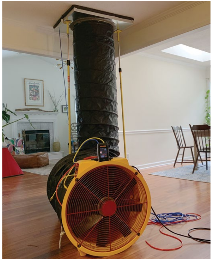
A blower door system used to test total system airflow at a main return.
