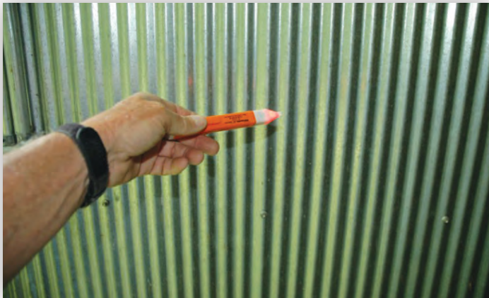
Metal siding energized in garage.
