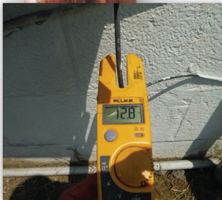
Lethal current (12.8) amps on GEC caused by a loose service neutral connection.
