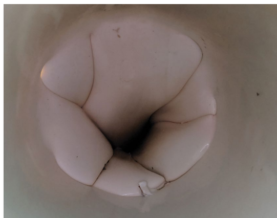
Photo 12. Results of flamethrower testing on a properly installed firestop collar.
