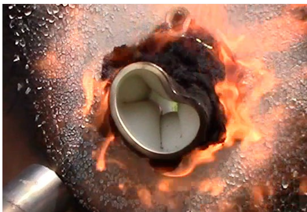
Photo 11. Testing on a properly installed firestop collar.
