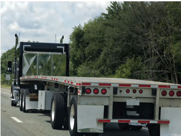
Photo 2. Example of camber on truck weight.
