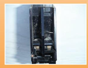
Photo 3. Older Bryant tandem breaker designed for two wires for each circuit.
