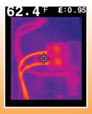
Photo 12. Thermal image of circuit under normal load.
