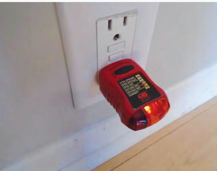
Photo 3. The trip button on a tester will not work if the circuit is ungrounded.
